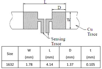
t: Copper foil minimum thickness of PCB
